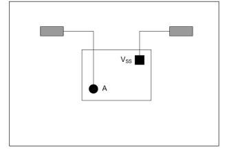
UHF transponders can be implemented using an EM4123 chip and an open dipole antenna.
